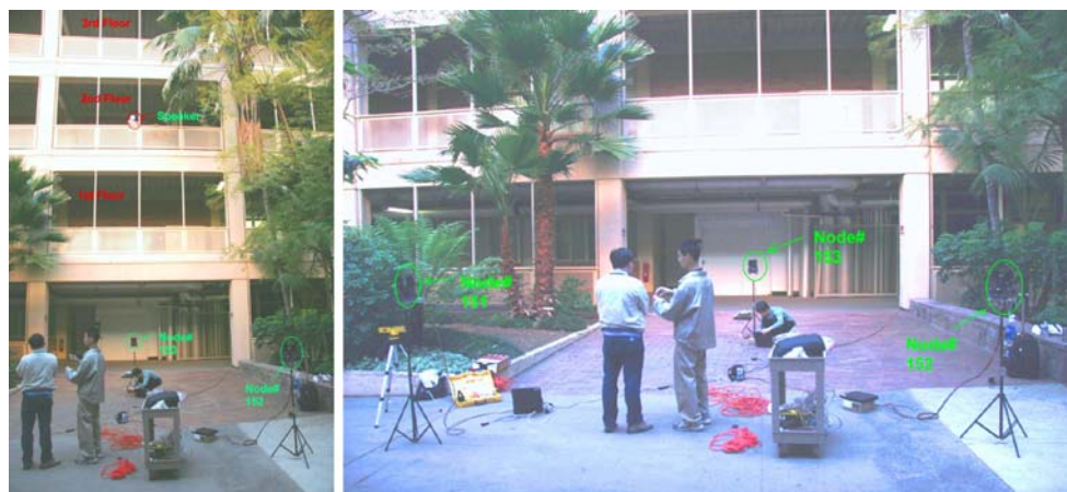
Figure 12 3D DOA accuracy testing experiment performed at the Boelter Hall in UCLA.
