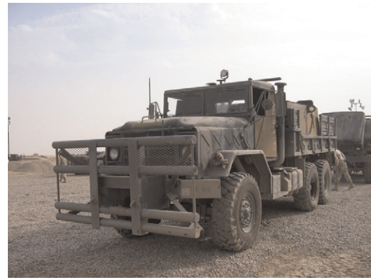
Figure 2 Operational adaptation on the battlefield. When US forces were caught off-guard by the development of improvised explosive devices (IEDs) in Iraq, active duty personnel up-armored their vehicles with whatever spare parts and scrap metal was available. It took years for the military to develop and deploy better-armored vehicles, but such hillbilly armor provided an interim solution. https://en.wikipedia.org/wiki/Improvised_vehicle_armour#/media/File:HillbillyArmor5tonCargo.jpg .
