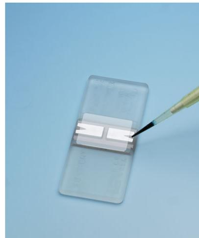
Figure 1: Hemocytometer loading guide.
